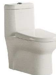
1689 Siphonic One-piece Closet Size: 700x375x720mm S-trap_300/400mm Roughing-in
