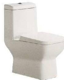
1685 Siphonic One-piece Closet Size: 650x360x760mm S-trap_300/400mm Roughing-in
