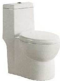
1659 Siphonic One-piece Closet Size: 675x340x730mm S-trap_300/400mm Roughing-in
