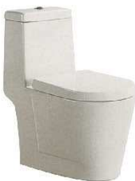
1672 Siphonic One-piece Closet Size: 660x370x760mm S-trap_300/400mm Roughing-in
