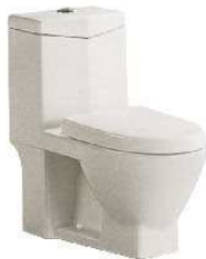
1606 Siphonic One-piece Closet Size: 510x260x510mm S-trap, 300/400mm Roughing-in
